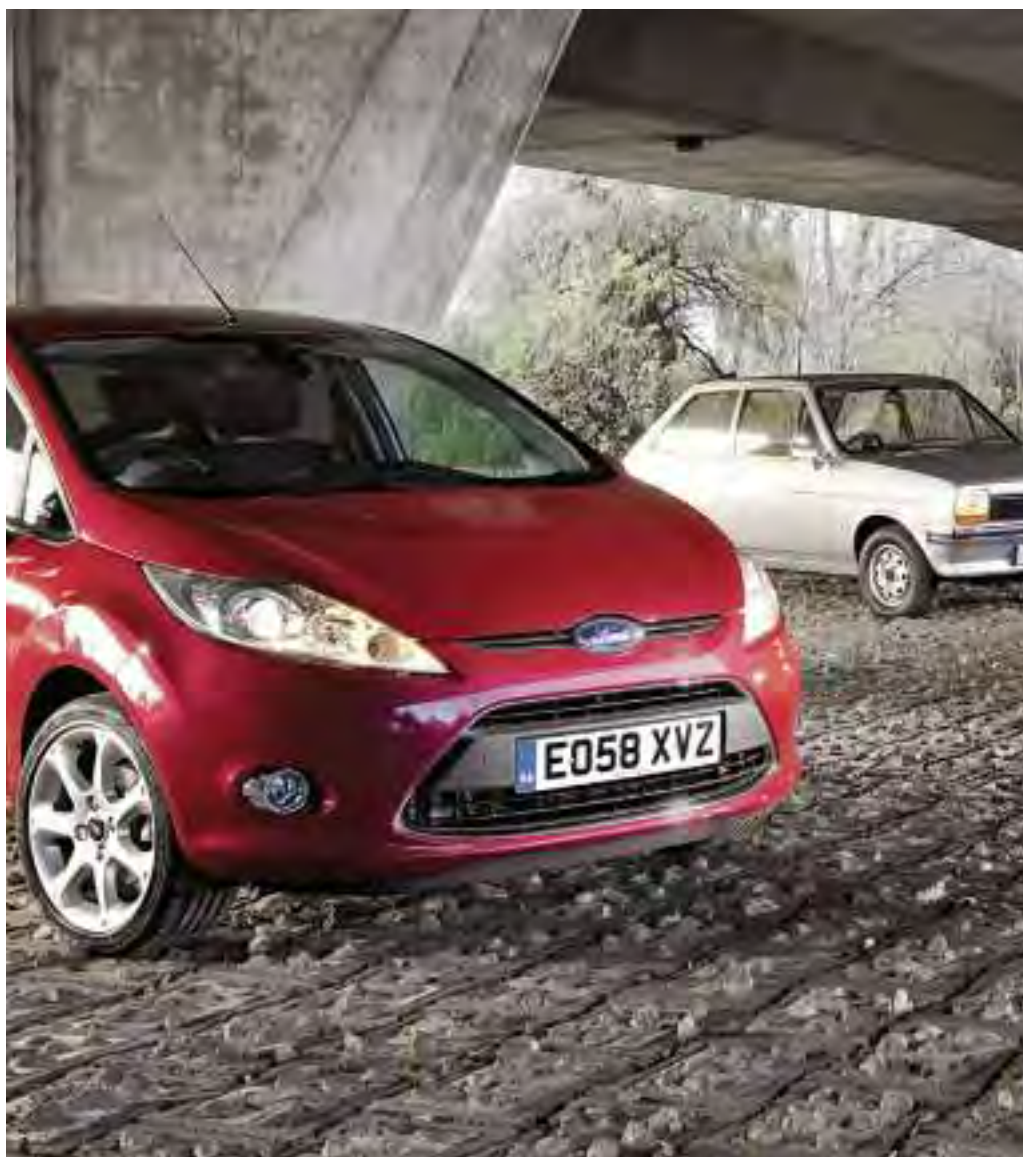
Mk1 Fiesta, 957cc, 48PS, 0 to 62 mph in 19.6sec, 35.5mpg, wheelbase: 2.286m, track 1.335m, overall length: 3.565m, width: 1.565m, weight: 730kg. From £1856 in 1977, equivalent to £14,020 in 2007 (based on average earnings)
